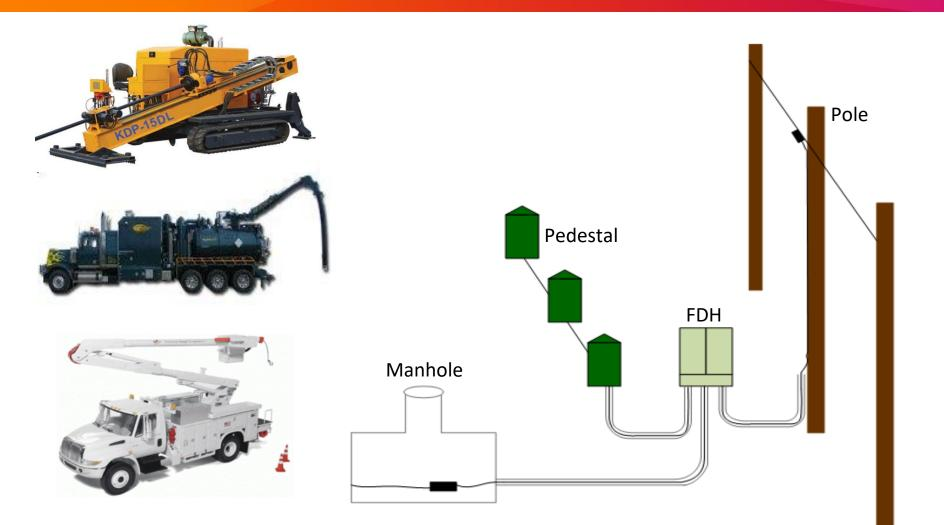
The placement of conduit and cable from our feeder network to each termination pedestal and pole.
